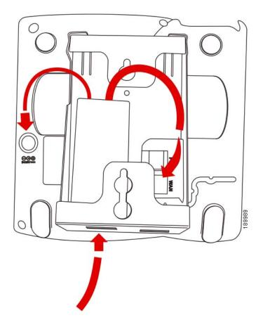
STEP 5 Hang onto screws mounted in the wall.
